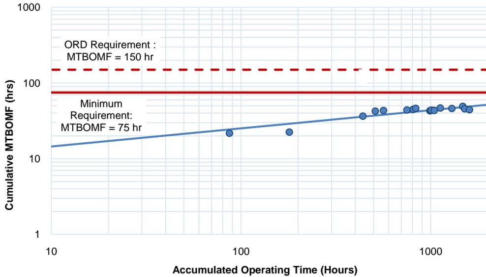
Figure 4. Duane Plot of RMS Test Data Since 2005
