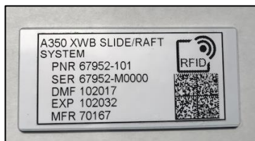
Figure 6 - AIT Integrated Data Plate Example
