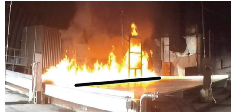
Fire on ILDFA Floor. 2022. Fuel Spill Fire Testing of an Ignitable Liquid Drainage Floor Assembly (ILDFA) for Chemical-Free Fire Control/Suppression, Air Force Civil Engineer Center, 2022, p.21.
